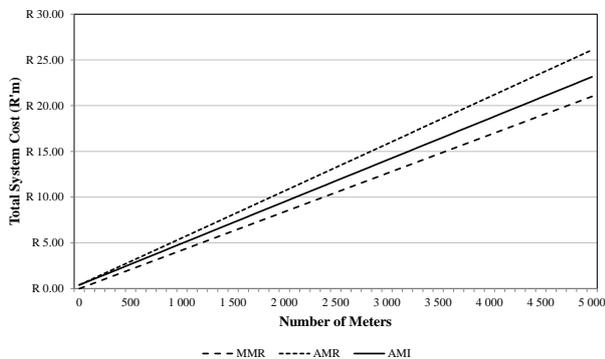
Figure 5: Comparison of platform costs for a three-phase system
