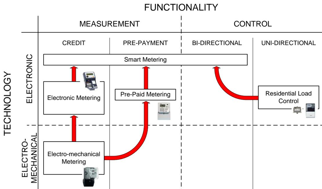
Figure 1: Overview of metering technologies in terms of functionality and technology base
